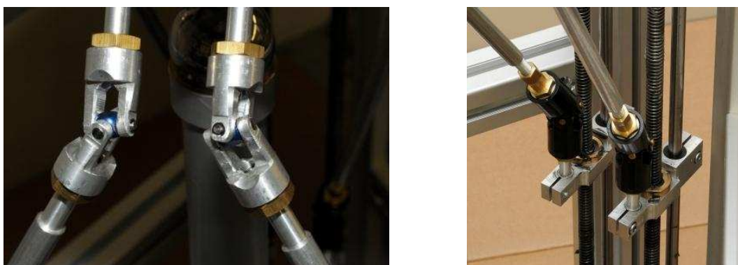
Fig. 4: Cardan joints at the upper (left) and lower ends of abutments (right)
