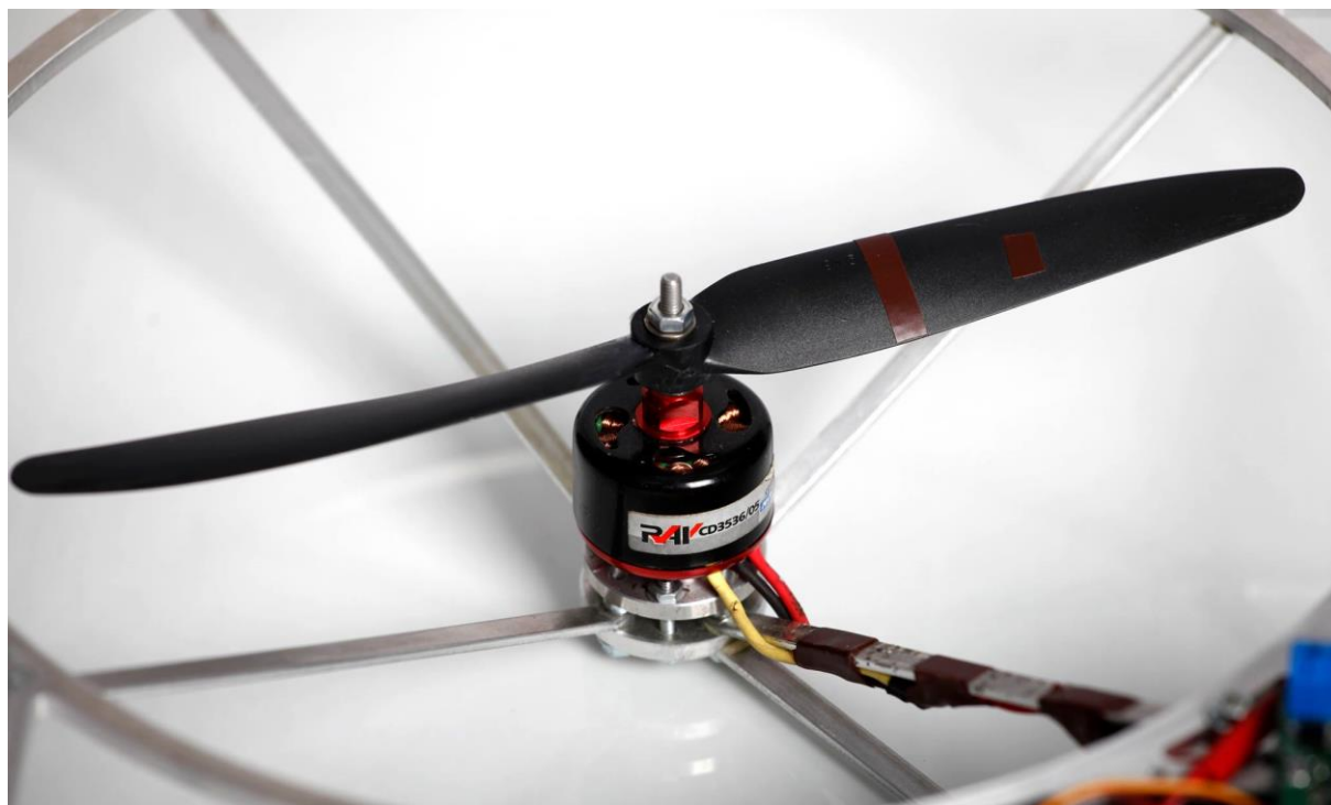
(Obr. 2.2) Motor RAY CD3635/05 s vrtulí
