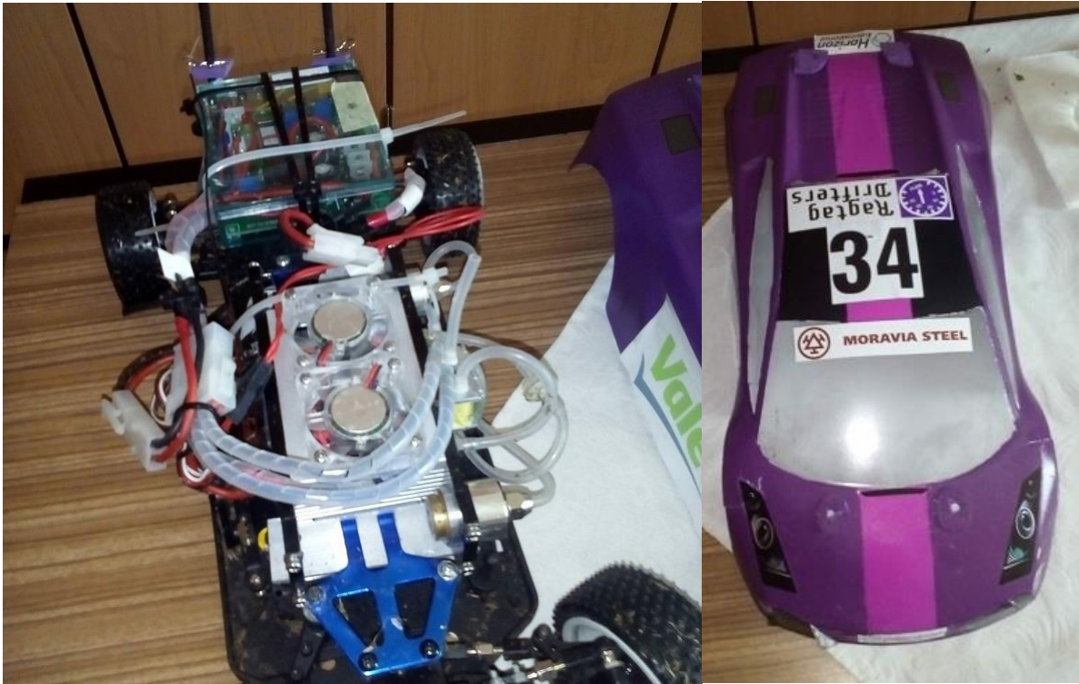
Fig. 3: left: finished assembly without the battery and Hydrostiks; right: decorated model shell
